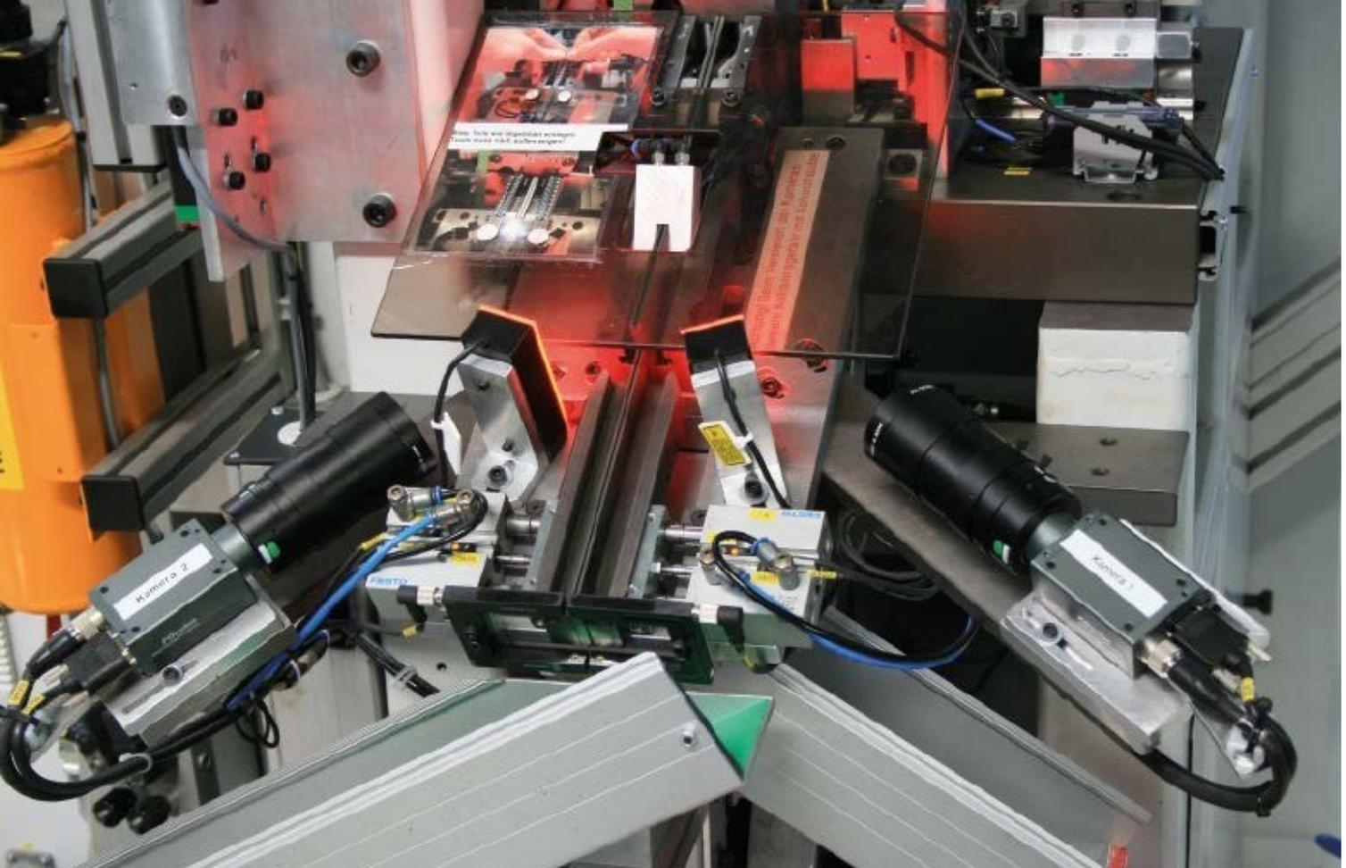
Practical example: Smart cameras can be used to extend existing PC-based vision systems.
